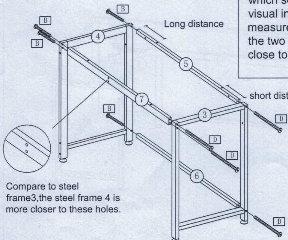
You may not be able to see which section is shorter by visual inspection. You can measure the distance between the two sides. The short side is close to the No. 3 tube.
