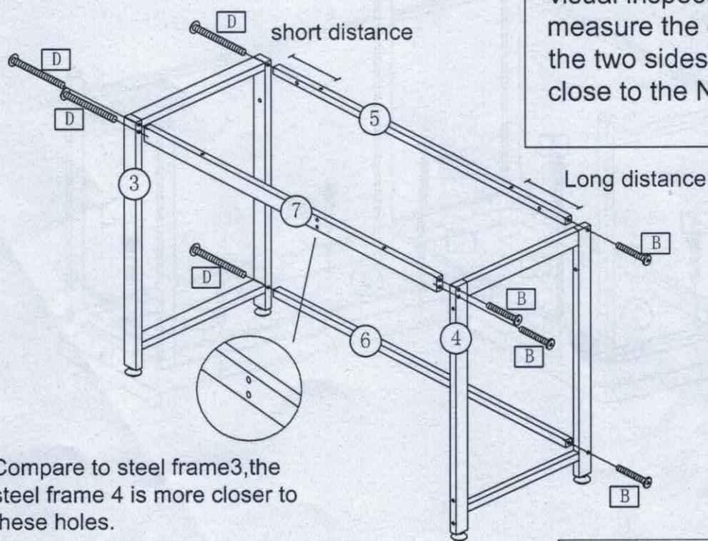
Compare to steel frame 3, the steel frame 4 is more closer to these holes.
